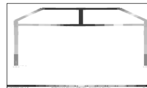
F24. Structure displacement diagram under dead load.
