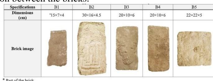
**Figure 4. Appearance characteristics of brick samples**
