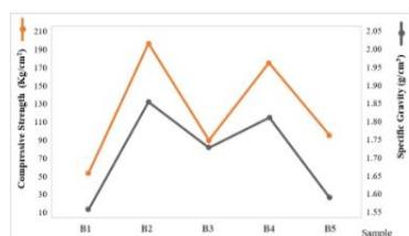
**Figure 5. Comparison of two graphs of compressive strength and specific weight of samples according to time period**
