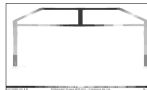
F24. Structure displacement diagram under dead load.
