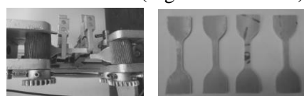
F18. Samples before and after testing (Razi Metallurgy Research Center).
