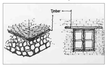
F13. Using wood in different parts of a house.
